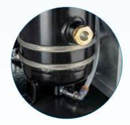
**Oil heater**Prevents intermittent-use condensation by maintaining a constant oil temperature while unloading/idle.
